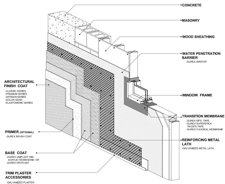
GALVANIZED PLASTER OR VINYL STOP CASING BEAD
