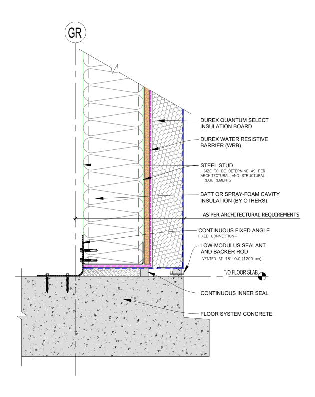
Durabond details are offered to assist in the development of project specific details. Design principles and variables incorporated in the final details and specifications are the responsibility of the project design professional.
