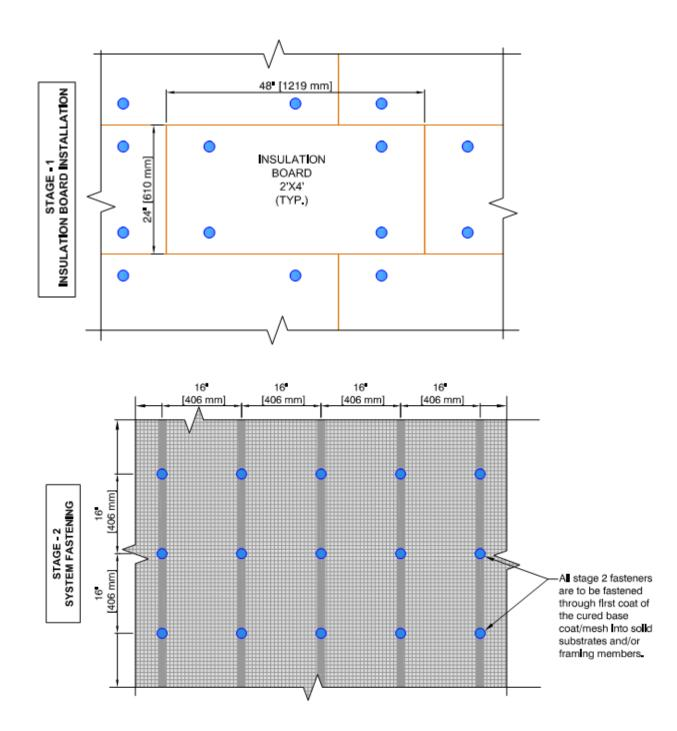
SPEC NOTE: The above fastening pattern addresses recommended fastener placement for typical wall installations. Consult Durabond Building Products Ltd. for project-specific installations.
