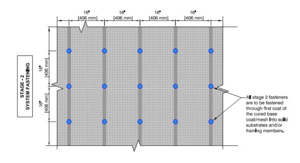
*SPEC NOTE:* The above fastening pattern addresses recommended fastener placement for typical wall installations. Consult Durabond Building Products Ltd. for project-specific installations.
