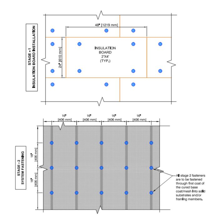
*SPEC NOTE:* The above fastening pattern addresses recommended fastener placement for typical wall installations. Consult Durabond Building Products Ltd. for project-specific installations.
